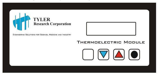
Access the automatic calibration function by turning off the main power using the rocker switch on the right rear panel. Depress all three of the labeled buttons on the front panel simultaneously, and turn the main power on *while keeping these switches depressed*. After characters appear in the LCD display, release the front panel buttons. The device will then enter auto-calibrate mode.
