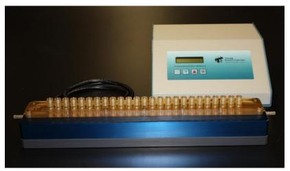
increments up or down. The setpoint is displayed on an LCD screen, along with the actual temperature and the power consumption of the driver circuit. An asterisk (\*) appears in the upper right corner of the screen when the temperature is in stable equilibrium.
